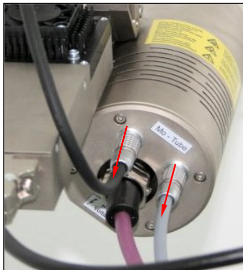
Fig. 43: Remove tube housing and filament cable
