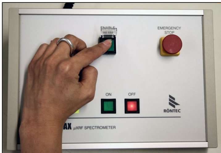
Fig. 35: Verification of the start with the "Enable Beam" button on the terminal
